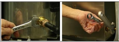
Tighten brass connectors
